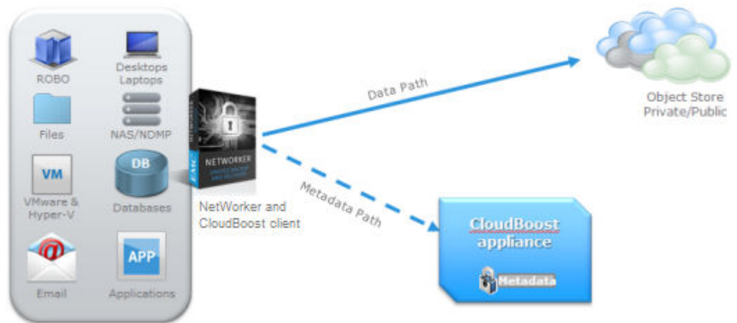
Figure 1 Clients backed up directly to the cloud
