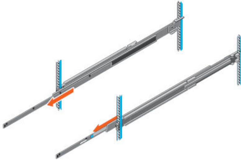
Figure 4 Pull the inner rails out of the cabinet
