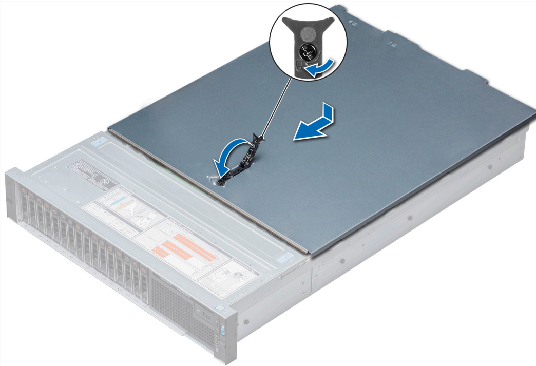
Figure 42 Remove the system cover
