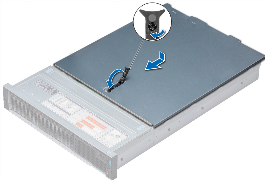
Figure 16 Install the system cover
