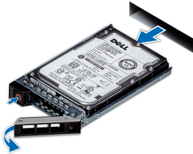
Figure 8 Removing a hard drive
