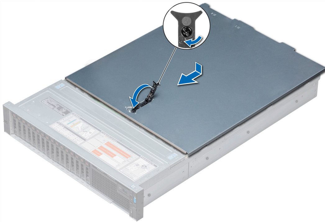
Figure 19 Removing the system cover
