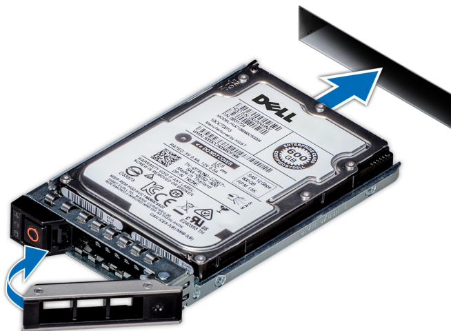
Figure 9 Installing a hard drive
