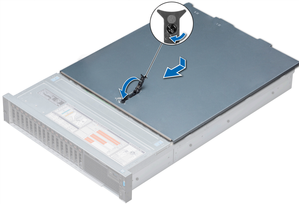
Figure 34 Remove the system cover
