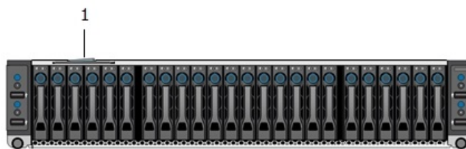
Figure 2. VxRail Appliance product serial number tag (PSNT) location (Models 60 through 280)
