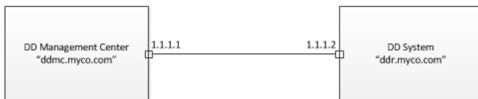
Figure 3 Simple case: DD Management Center connecting directly to a Data Domain system
