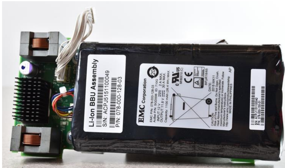
Figure 5. Battery Backup Unit
