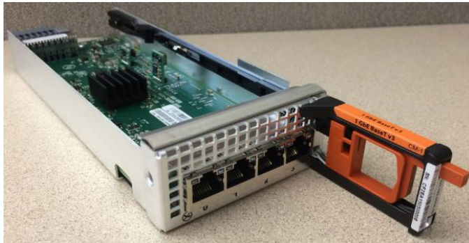
Figure 13. 1GbE BaseT I/O Module
