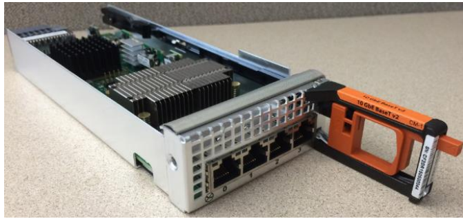
Figure 12. 10GbE BaseT I/O Module
