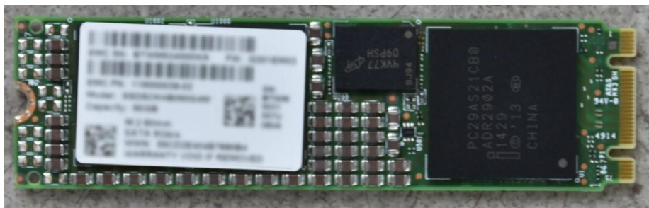
Figure 5. M.2 SSD Device
