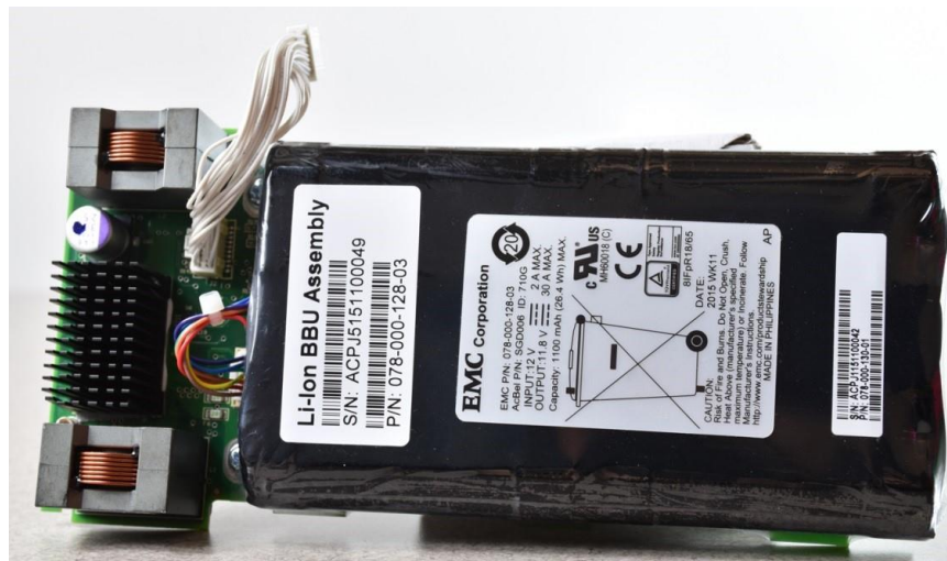
Figure 7. Battery Backup Unit
