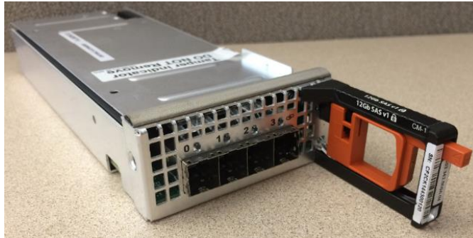
Figure 10. 12Gb SAS I/O Module
