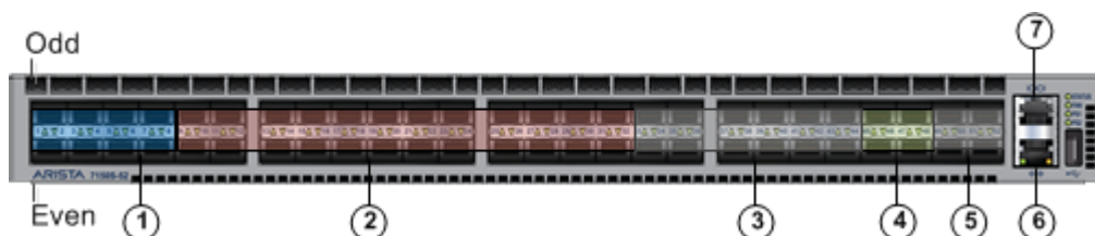
Figure 13 Arista 7050S-52 ports
