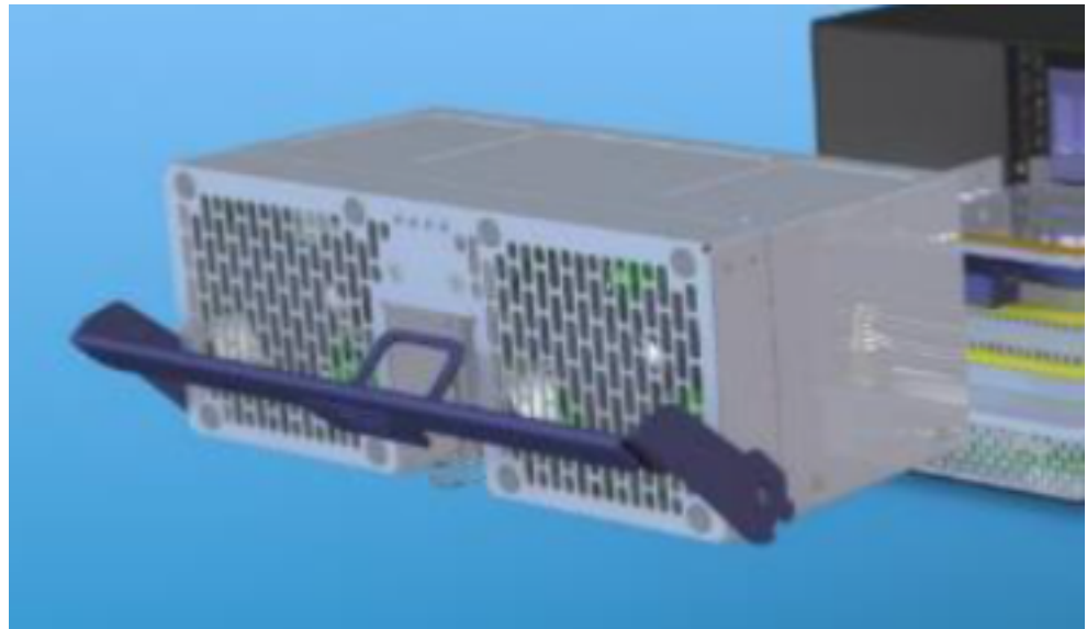
Figure 26 Power supply separated from I/O module
