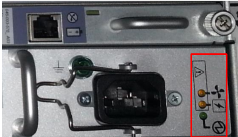
Figure 4 Power Supply A LEDs
