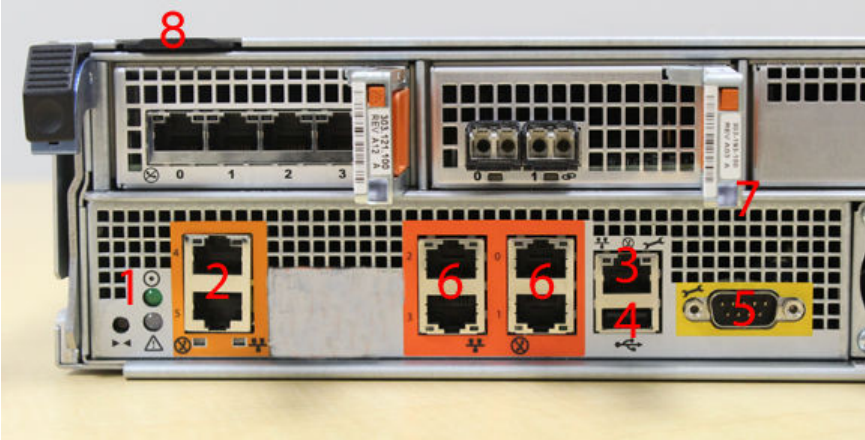
Figure 7 Onboard interfaces and SN tag for the DD2500 system
