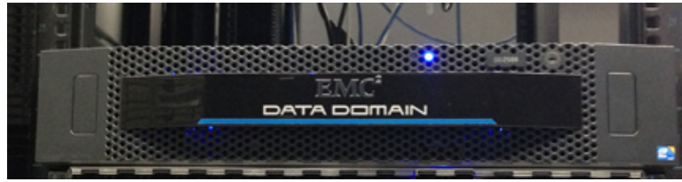
Figure 3 Bezel showing lighted system power LED
