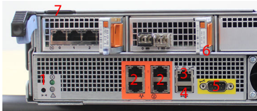
Figure 8 Onboard interfaces and SN tag for the DD2200 system
