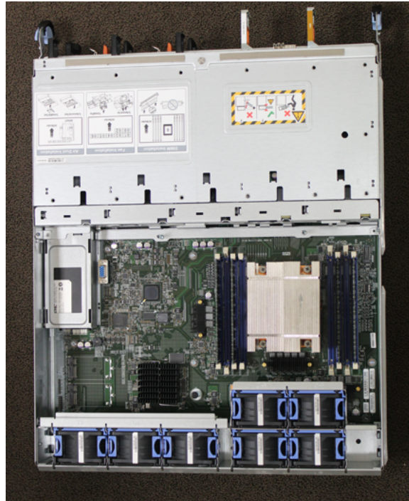
Figure 11 Top view of SP module with air duct removed (DD2200 system shown)
